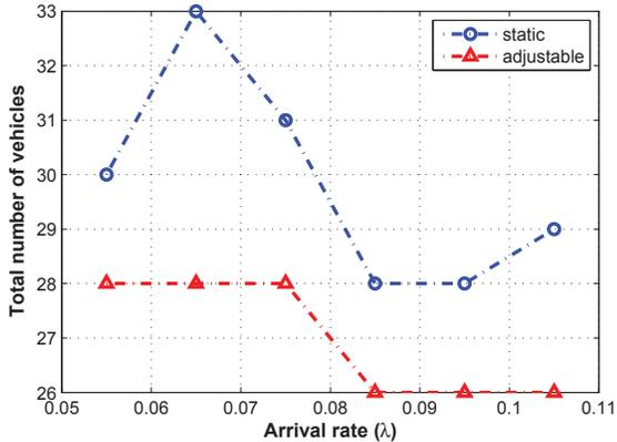
Fig. 9: The minimum number of vehicular cameras required by arrival rate
