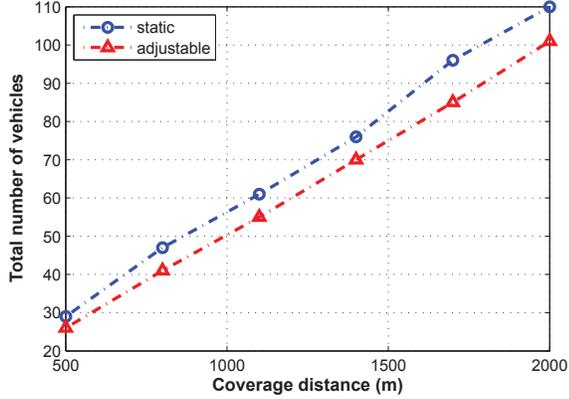
Fig. 8: The minimum number of vehicular cameras required by coverage distance
