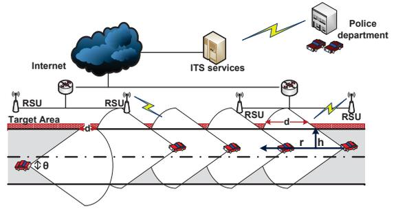
Fig. 2: Network model for barrier coverage in VANETs
