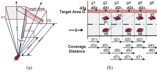
Fig. 6: Barrier coverage with adjustable vehicular camera
