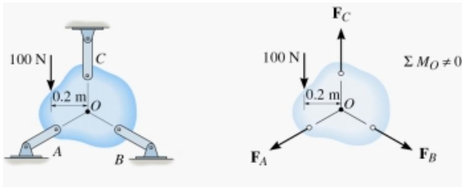
In 3D problems like this, the support reactions all **intersect a common axis**, so the constraints are improper. Constraints A and B are not proper, since they do not resist the moment caused by 400N force.
