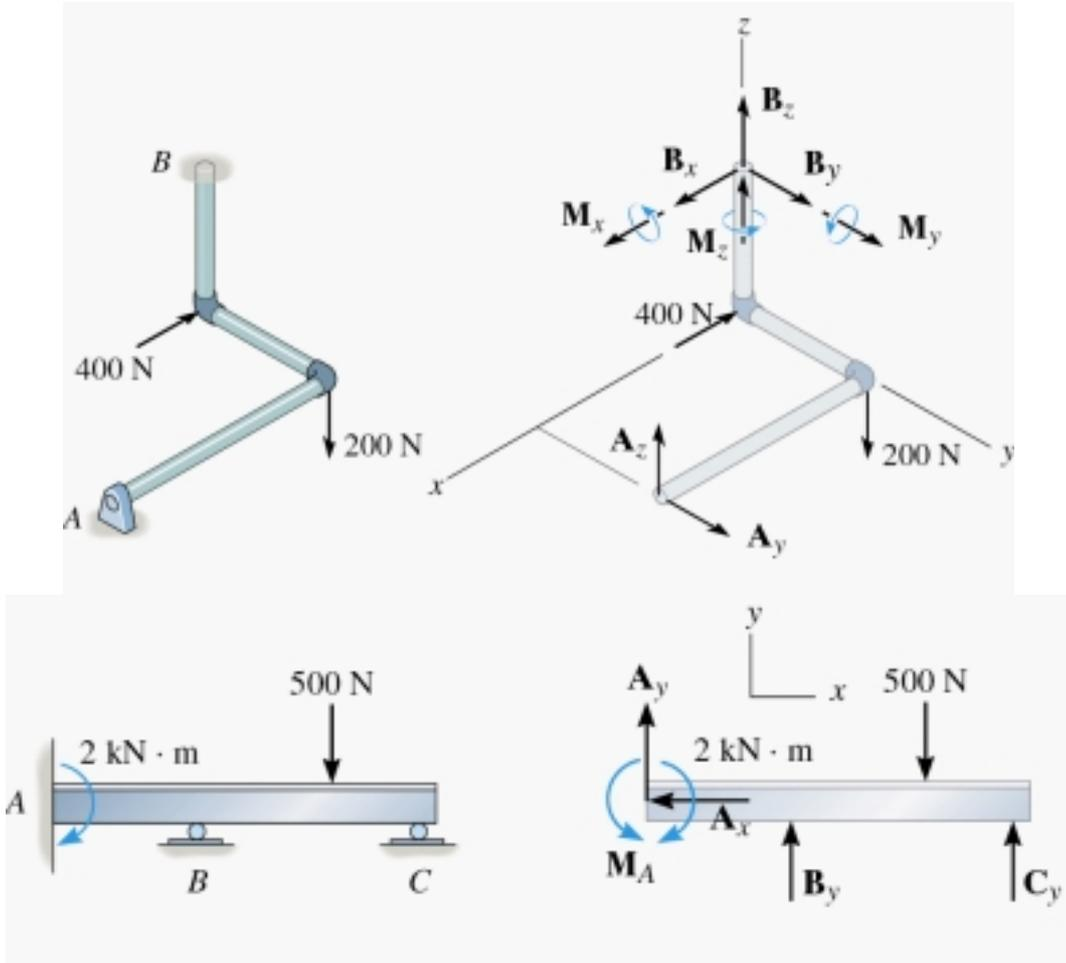
When there are fewer reactive forces than the equations of equilibrium, they constraints are called **Partially Constrained**.
