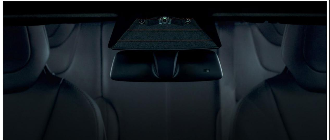
**Fig. 1.5: Front-facing Portion of Tesla Autopilot System**
