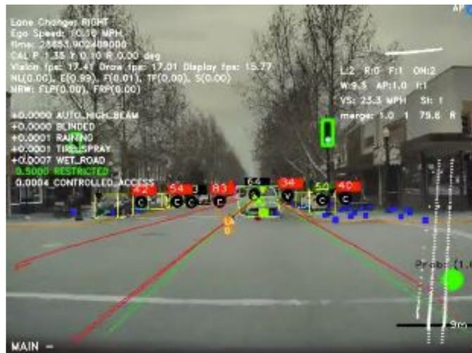
**Figure 1: Tesla's Neural Networks displaying live object semantic segmentation, object detection and monocular depth estimation for its Autopilot AI (Tesla, 2020)**
